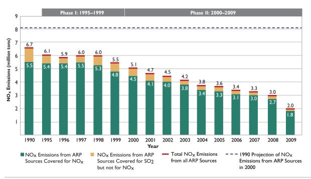
Figure 2-3. NO<sub>x</sub> emission levels for all ARP sources, 1990 to 2009 (U.S. EPA, 2010b).
