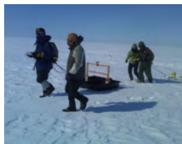
GEOPHYSICS: Exploring subsurface characteristics using ground-penetrating radar.
