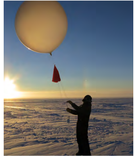
Launching an instrumented balloon to collect weather information. Photo: Kevin Hammonds
