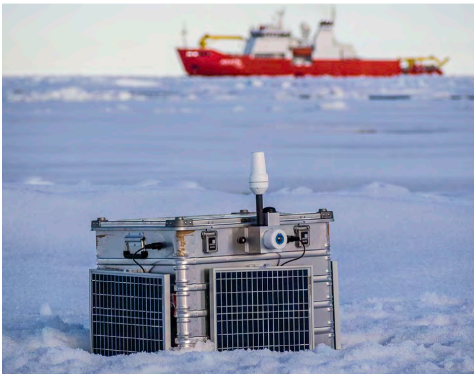
A wave buoy sits on the sea ice. It was deployed from the R/V Araon (in the background) of the Korea Polar Research Institute (KOPRI). Photo: Martin Doble (Villefranche Oceanographic Laboratory, France)
