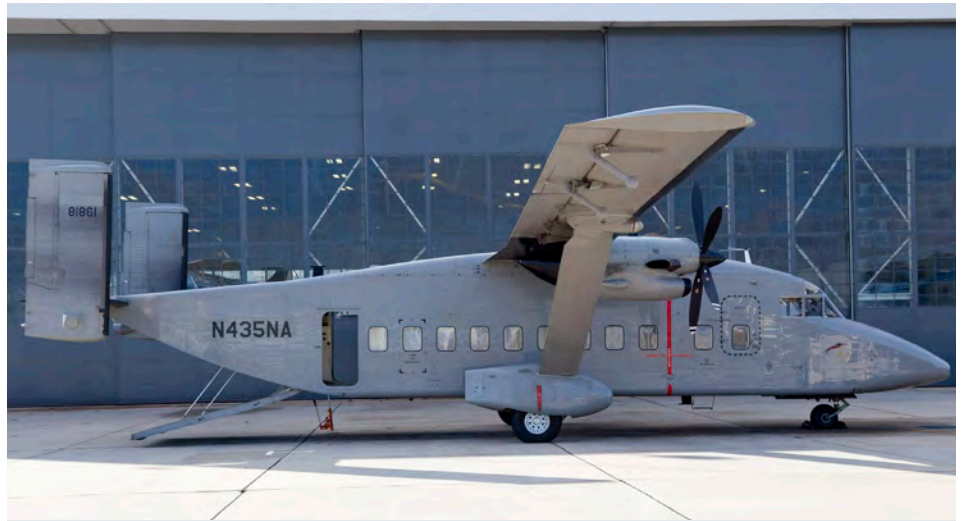
CARVE uses instruments aboard a NASA C-23 Sherpa aircraft to measure air and surface conditions and concentrations of greenhouse gases (carbon dioxide, methane, etc.). See page 17 for a description of the CARVE field campaign. Photo: NASA/Wallops
