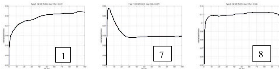
Figure 6 Examples of typical friction-slip curves for tyres number 1, 7 and 8.
